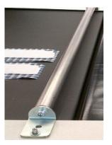
This very high power magnetic bar, allow to stop any metalic object that may enter in the fusing machine.
