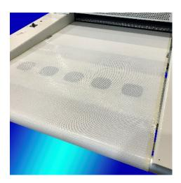
Active cooling system is a powerful active cooling exit belt made in open mesh material that allow air circulation, inside the belt are placed cooling fans
