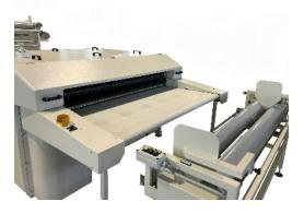
Our Laminating system can be equipped with: 3 Position Unwinding = FABRIC + FILM + FABRIC
