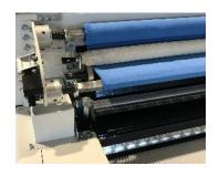
Programmable movement belt cleaning device with fabric collection
